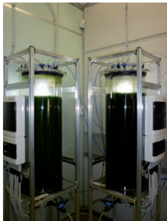
Fig. 2 Desmodesmus communis cultivation in 70 L photobioreactors.
